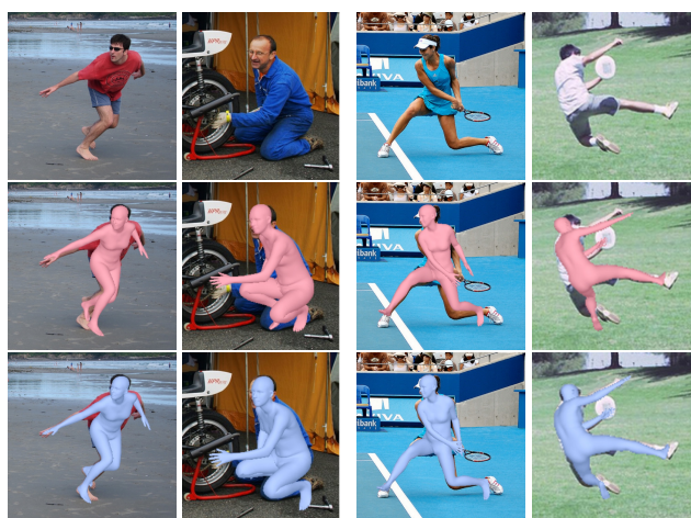
Figure 9. Refinement in-the-wild . Examples from the coco validation set. From top to bottom are images, predictions without refinement update ( T=0 ), and predictions from ReFit ( T=5 ).
