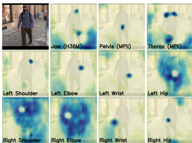
Figure 8. Per-keypoint feature map . Each channel corresponds to the learned features of a keypoint. Here we show feature maps from the semantic keypoint model. The network learns a peak (blue) or a valley (yellow surrounded by blue) response around the keypoint, without direct supervision.
